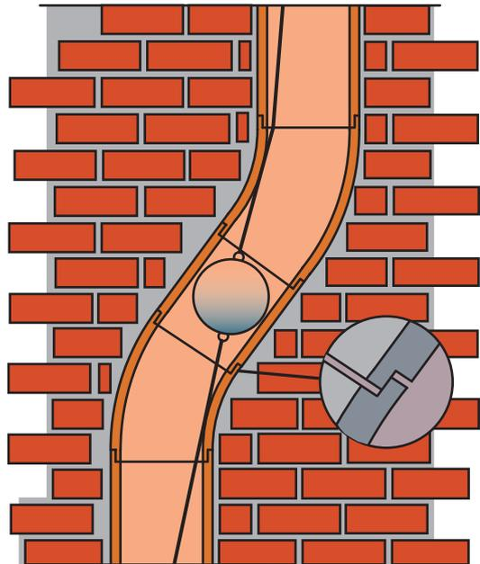
The space between the outside of the flue liner and the chimney stack should be filled with insulating material such as a weak lime mortar or lightweight insulating concrete.
