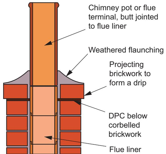
A tapered terminal should be fitted over the last liner as shown below. Note that the top of the last liner lies within the corbelled brickwork in this case.
