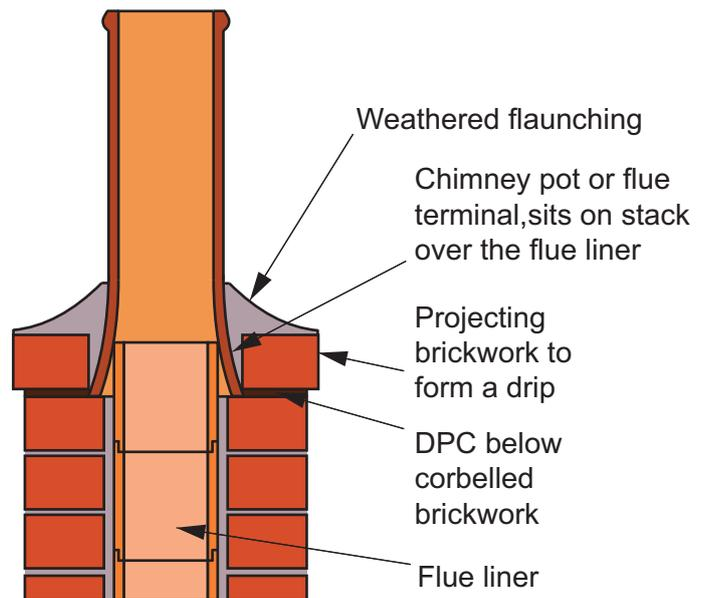
A terminal may be formed by extending the flue liner to project above the top of the stack as shown below. It is recommended that at least 150 mm projects above the flaunching.
