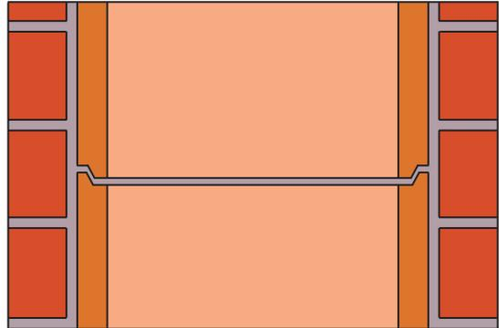
The joints between liners must be made with a fireproof mortar or manufacturer's proprietary fireproof sealant.
