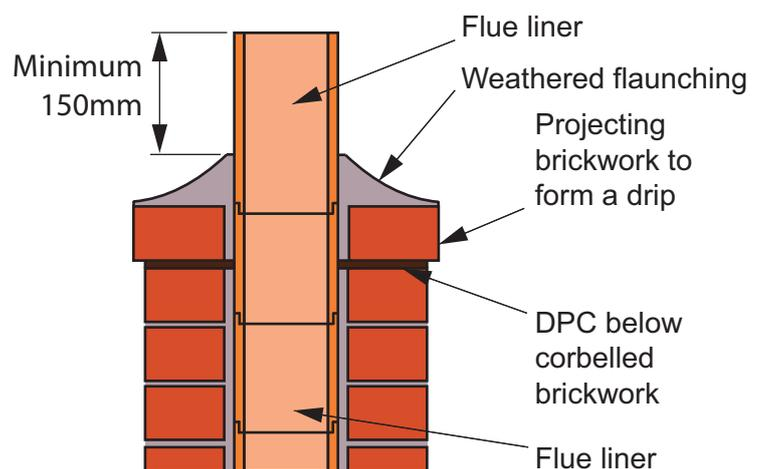
A flue terminal should always be used to obtain a satisfactory chimney performance. The chimney should not be terminated with just a mortar flaunching.
